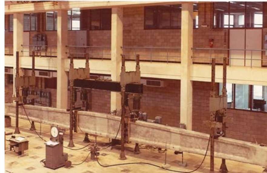
Failure test roof beam after repair
