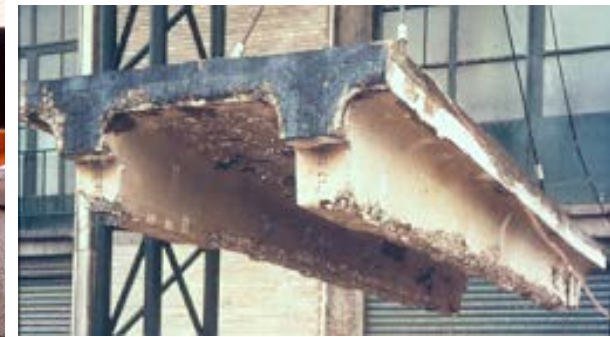
Failure test roof beam after repair
