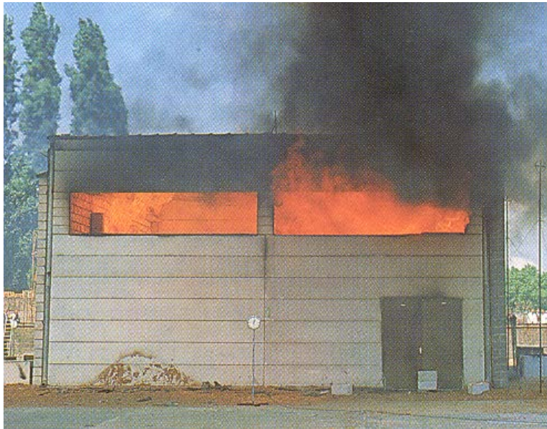
Test on precast industrial hall
