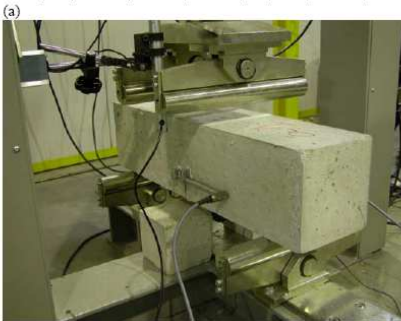
Figure 4. UNI test: (a) geometry and test set-up; (b) specimen image during testing.
