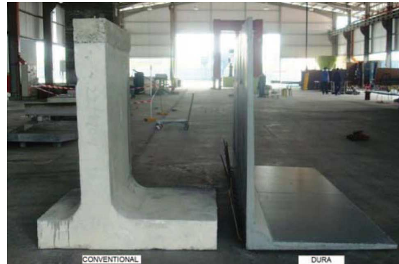
Solution in conventional concrete and UHPFRC ( f_{cm} = 160 \text{ N/mm}^2 )
